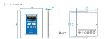
\*For details on the detection section and calculation display section, please refer to pg. B14-B15.
